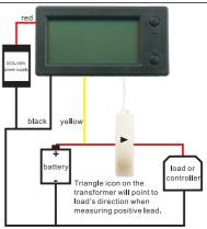
The above pictures show the wiring method for those that charging port and discharging port are the same one. If they don't share the same port, you need to make the positive of charging cable go through the hole of transformer.
