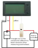
When the measured voltage is over DC 5-90V, this meter must be connected with three-wire system connection. A separate power supply is needed for this meter. As the following picture shows:
